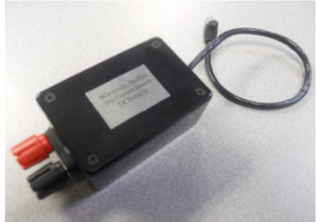
Figure C.9 - Dry Contact Sensor
