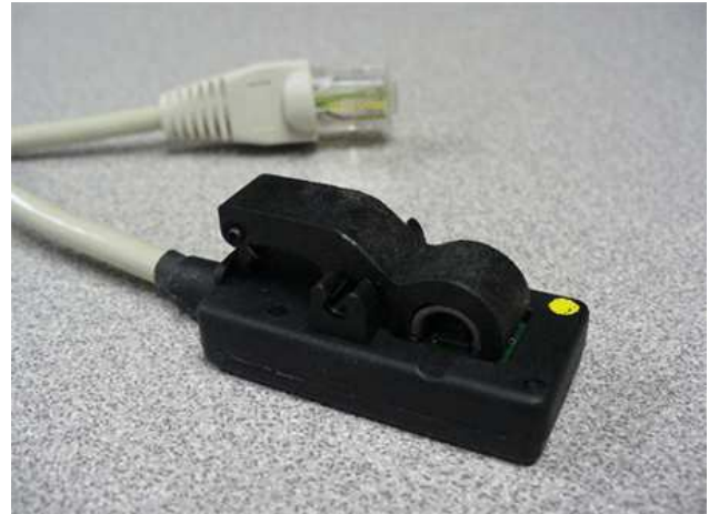
Figure C.2 - Clothespin Current Sensor
