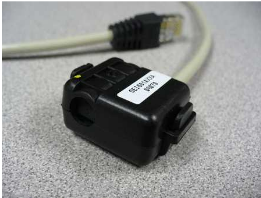
Figure B.3 - Clamshell Current Sensor (Model# CS-HE-CS)
