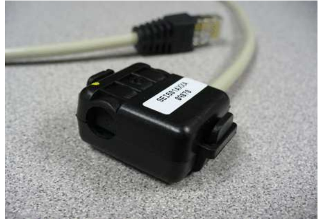
Figure C.3 - Clamshell Current Sensor
